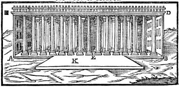
This figure is made voushout voull or porch, that the order of the pillars voithin might be seene. AB The length of an hundreth cubites. BC The breadth of fiftie. BD The height of thirtie. EFGH The source of pillars. I The three rouves of voindouves. K The porch or gallerie before the house.
